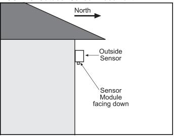
Mount the outside sensor with the sensor module facing down to prevent accumulation of dirt or water.
